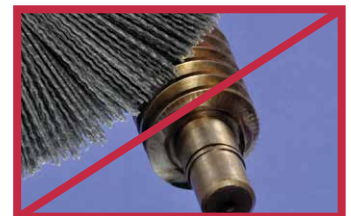
INCORRECT Point of Contact
