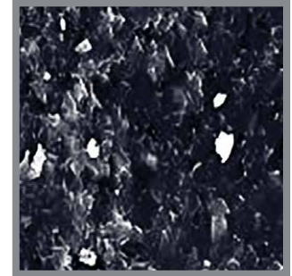
Fractured 321 Grain (Courtesy of 3M™)
