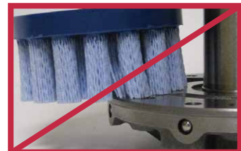
INCORRECT Point of Contact
